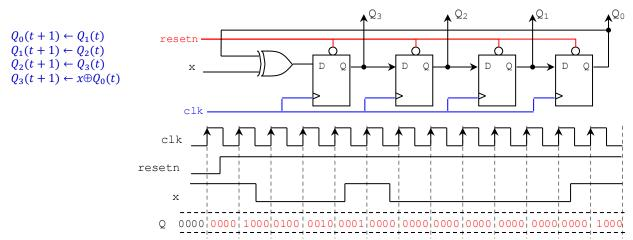
• Complete the timing diagram of the circuit whose VHDL description is shown below. Also, get the excitation equation for q.
