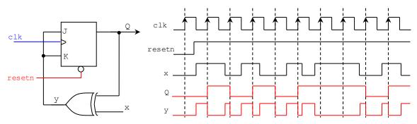
• Complete the timing diagram of the circuit shown below: (6 pts)
